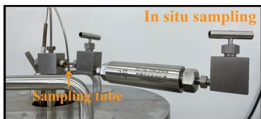
Figure 2: In-situ sampling method.
