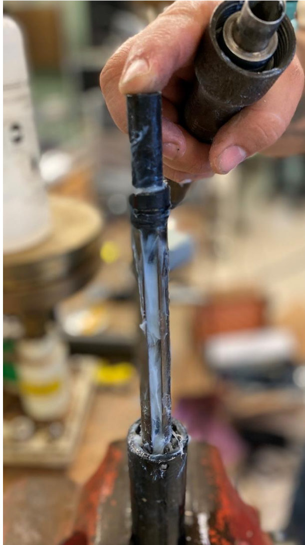
Figure 3: Interior of cable head used to transition from the cable to the tool is filled with grease to temporarily prevent fluid contacting the electrical conductors.
