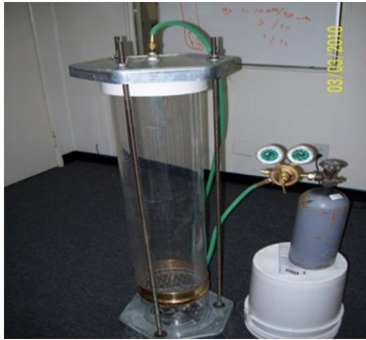
Figure 9: Vugular lost circulation testing apparatus, with variable screen opening sizes to simulate large vugs or fractures
