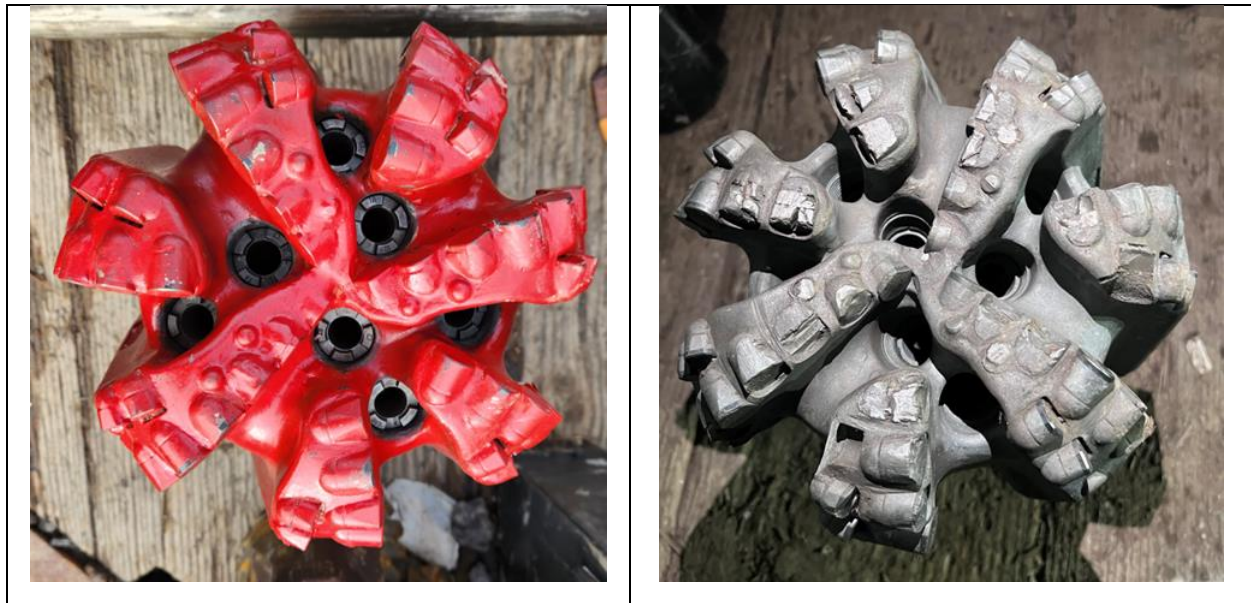
Figure 21. Bit 12 pre-drill (left) and post-drill (right) photographs.
