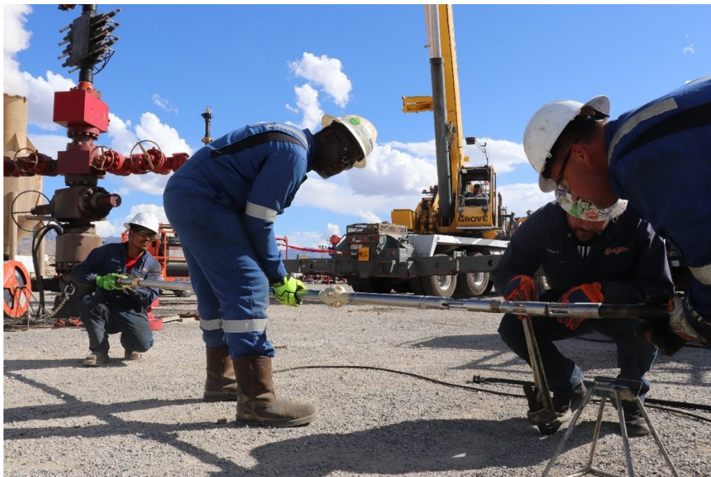
Figure 10: Full chemical tool assembly attached to weight bars and being loaded into lubricators.
