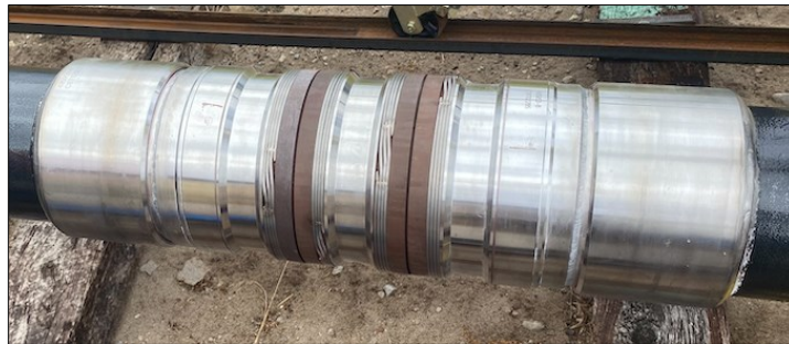
Figure 1. HPHT packer from Welltec Inc. Packer capable of withstanding 320°C and designed to expand and set at 6,000 psi with a maximum run in hole ID of 8.42” (Álvarez et al., 2024).
