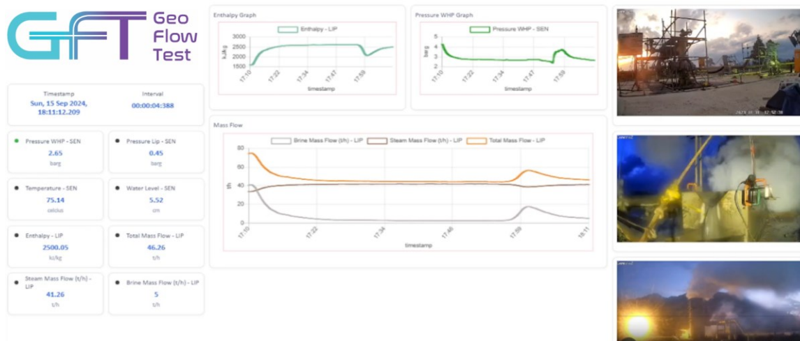
Figure 14. Real-time data and visualization of Geoflowtest web-based dashboard during well production testing TLG-B.
