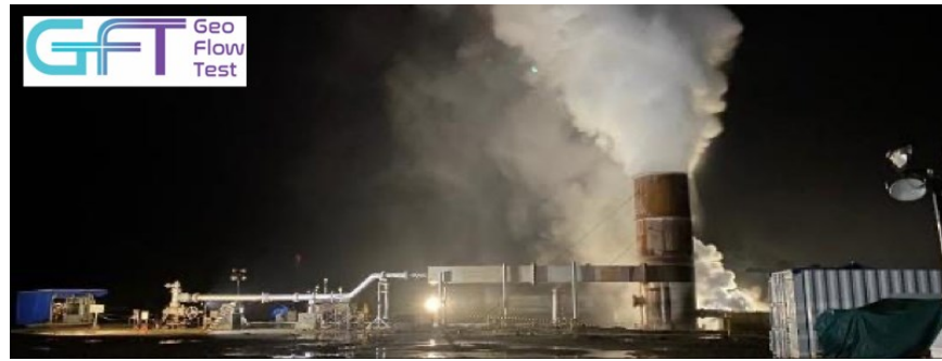
Figure 12. A photograph of lip pressure production testing at Ulubelu field using Geoflowtest device.
