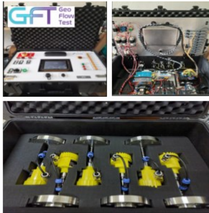
Figure 11. Protected modular housing and enclosures design of Geoflowtest.
