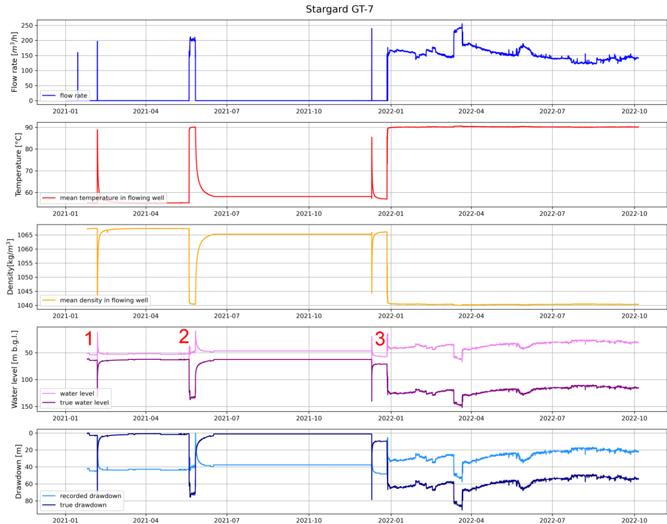
Figure 2: Effect of applying Thermalift calculator to exemplary dataset from sedimentary reservoir in Poland.
