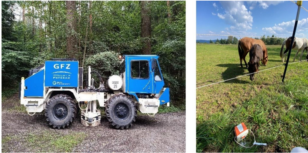
Figure 3: Seismic vibration source vehicle Inova Univib and Sercel Wings seismic recorder used in the first seismic campaign.
