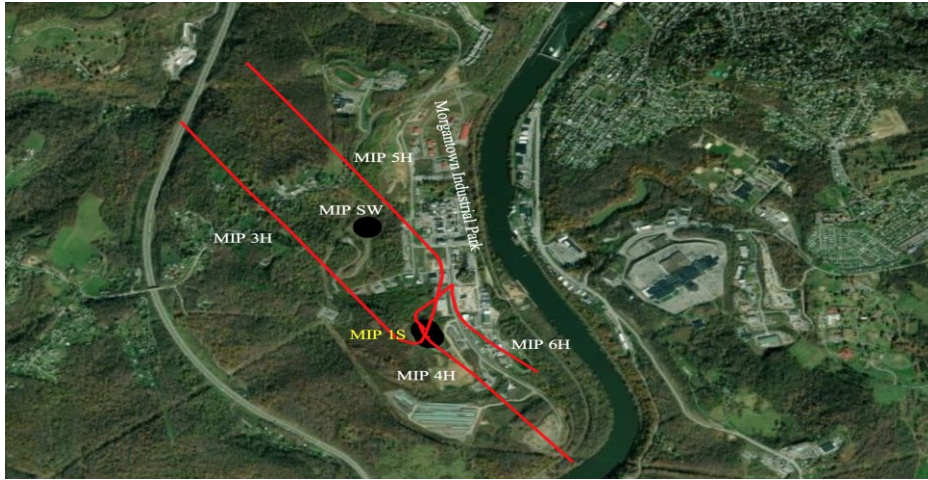
Figure 3: MIP Pad and 6 wells drilled and completed including MIP1S geothermal science well along with MIP 3H, 4H, 5H, 6H and SW. (Fathi et al 2024)
