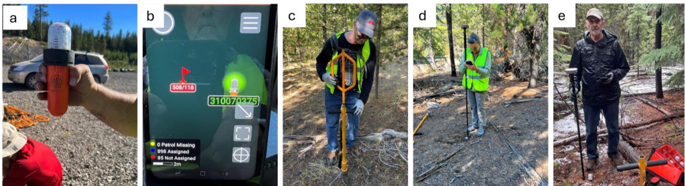
Figure 8. (a) A NuSeis seismic receiver: GPS, computer, battery, vertical geophone. (b) Handheld station locator and directions. (c) Slide hammer for punching secure receiver hole. (d) registering installed receiver at base of GPS guide pole. (e) Retrieval: GPS guide pole, map directions handheld cell phone, 10 station carrying sack.
