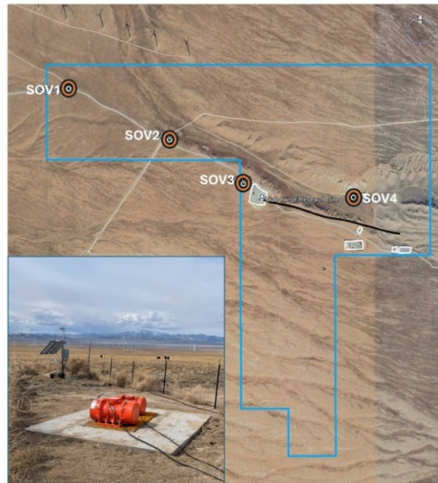
Figure 1: FORGE Utah field site in Milford, Utah. Orange circles show the location of the SOV sources; the injector well 16A is outlined in black; Utah FORGE Research Site is outlined in blue. In the left bottom corner, the figure shows a photo of an SOV location after installation where two motors were installed on a concrete pad.
