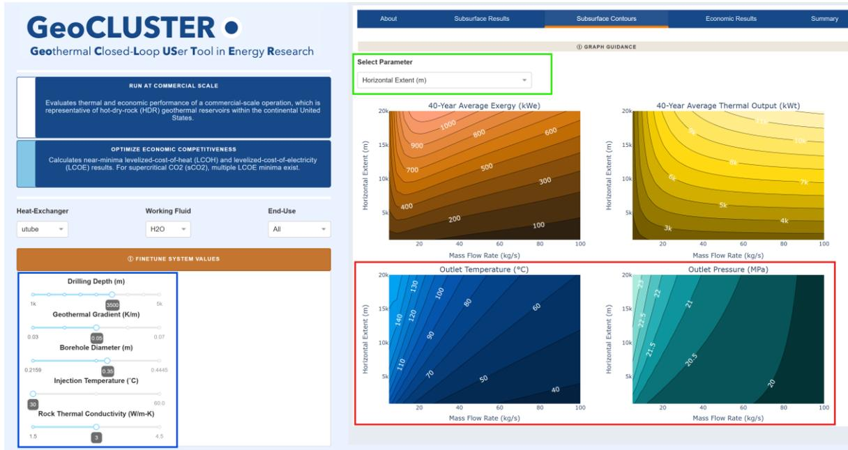
**Figure 5. Subsurface contours with parameter second parameter in green, variation of outlet state with respect to mass flow rate and second parameter in red, and parameters held constant in blue.**
