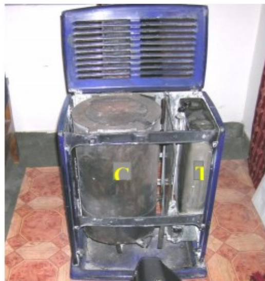
Figure 11. A typical "Bukhari" traditionally used in leh for space heating during winter.
