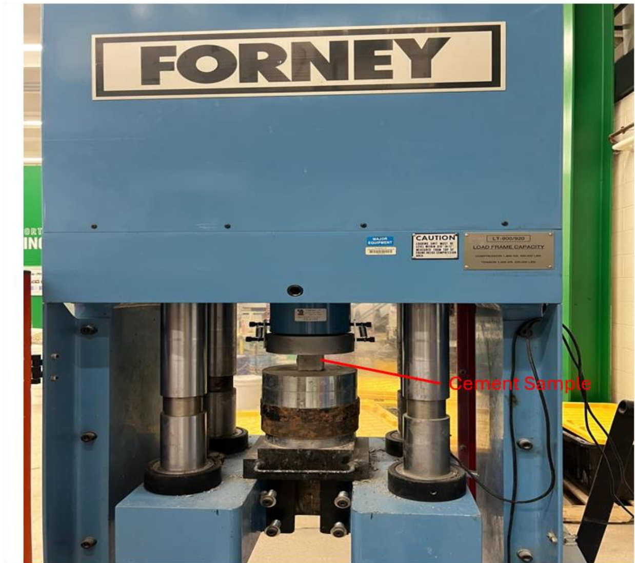
Figure 3: Compressive Strength test was performed on cement samples at curing temperatures using Forney 920 Series Universal Testing Machine.
