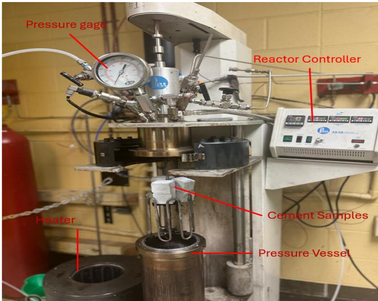
Figure 1: The autoclave reactor used to cured the cement sample, simulating geothermal well condition (Aluah et al 2024a).
