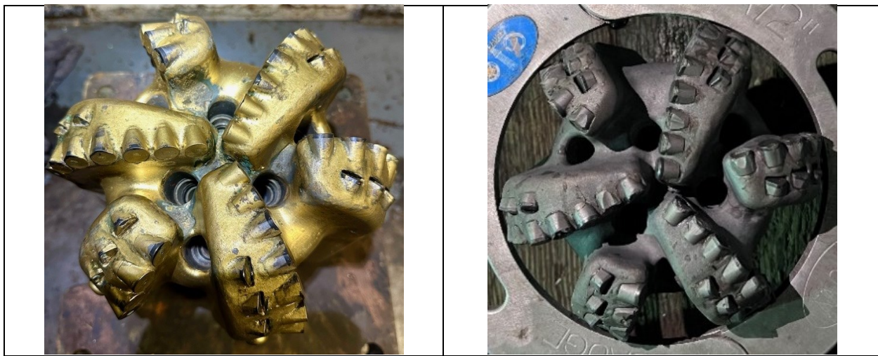
Figure 17. Bit 20 before (left) and after (right).
