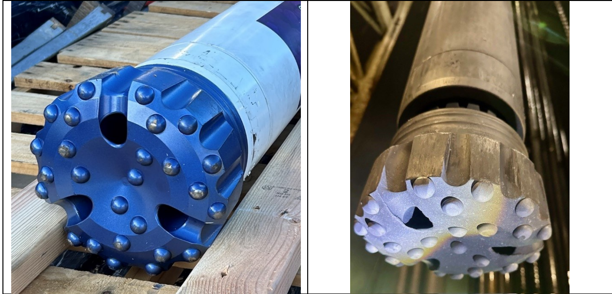
Figure 19. Percussive hammer (DTH) before (at left) and after drilling 40ft (at right).
