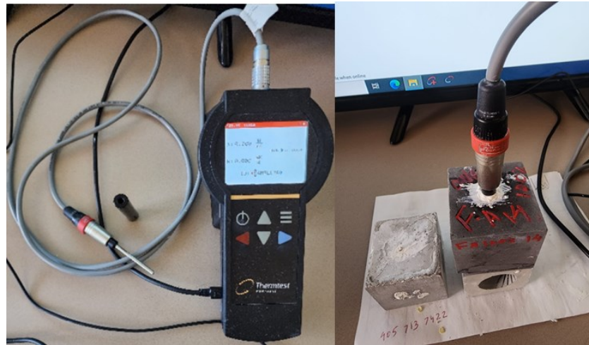
Figure 3: Measurement Platform –2 (MP 2) for the measurement of the thermal conductivity of the sample
