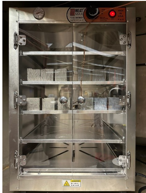
Figure 3 Heating environment for monitoring thermal cracking of geopolymer samples
