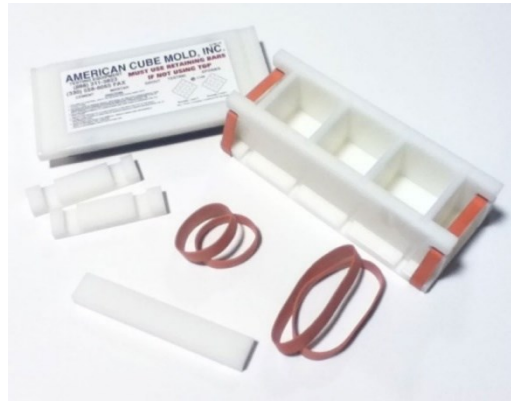
Figure 2 Plastic molds used to cure all geopolymer samples
