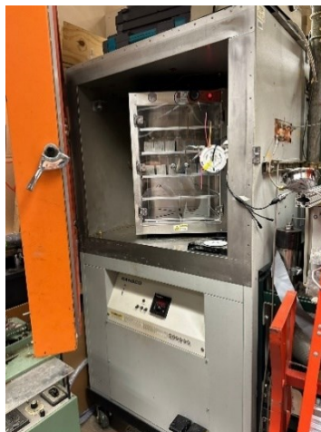
Figure 8 Larger oven used to house the entire experimental setup
