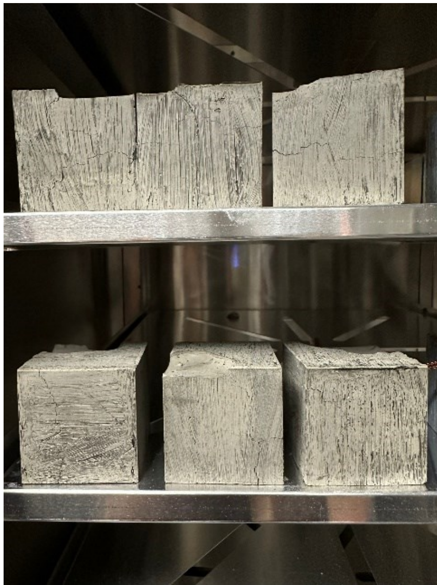
Figure 9 Neat geopolymer samples after 2 days in heating conditions, note thermal cracking on all 6 samples
