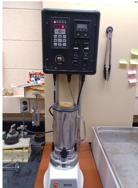
Figure 1 API Blender used to prepare all geopolymer slurries
