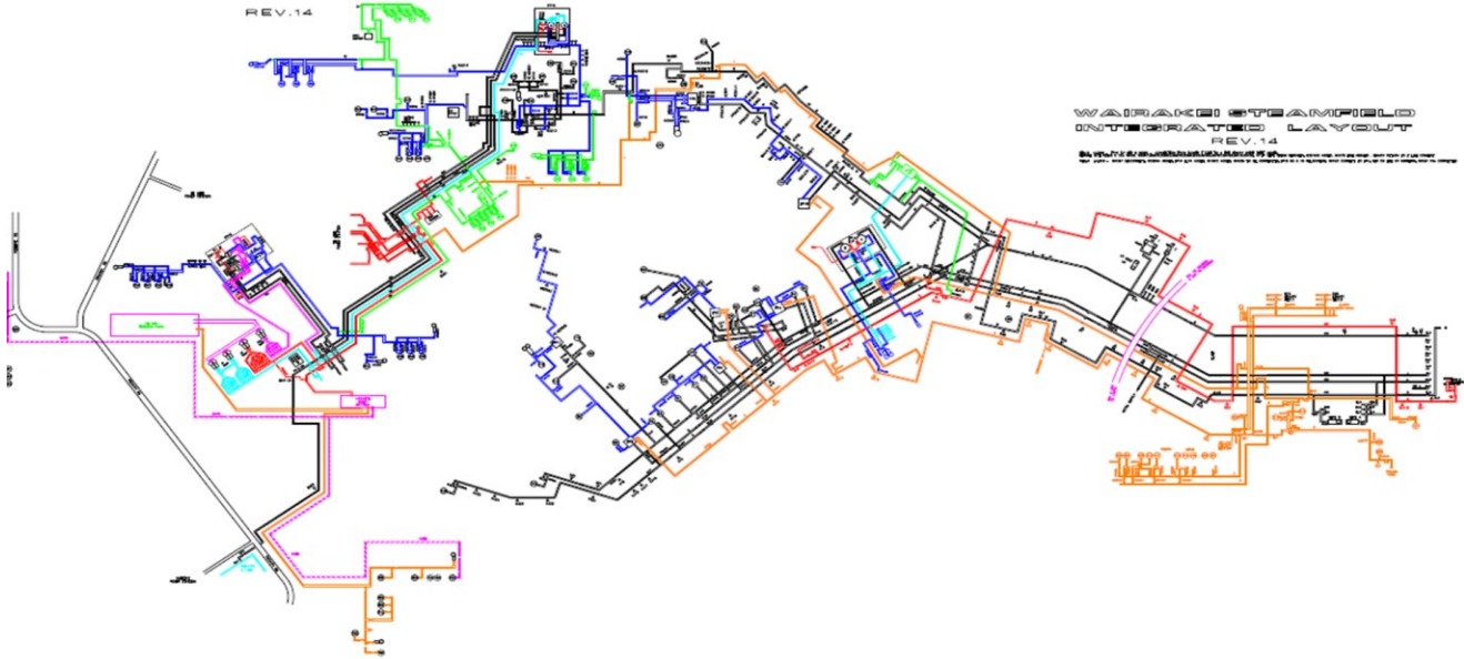
Figure 1: The layout of the Wairakei (Contact Energy) steam field, the basis on which we have developed the GOOML digital framework. This diagram illustrates the complexity of a steam field with dozens of wells, kilometres of pipelines, and several power generating stations.
