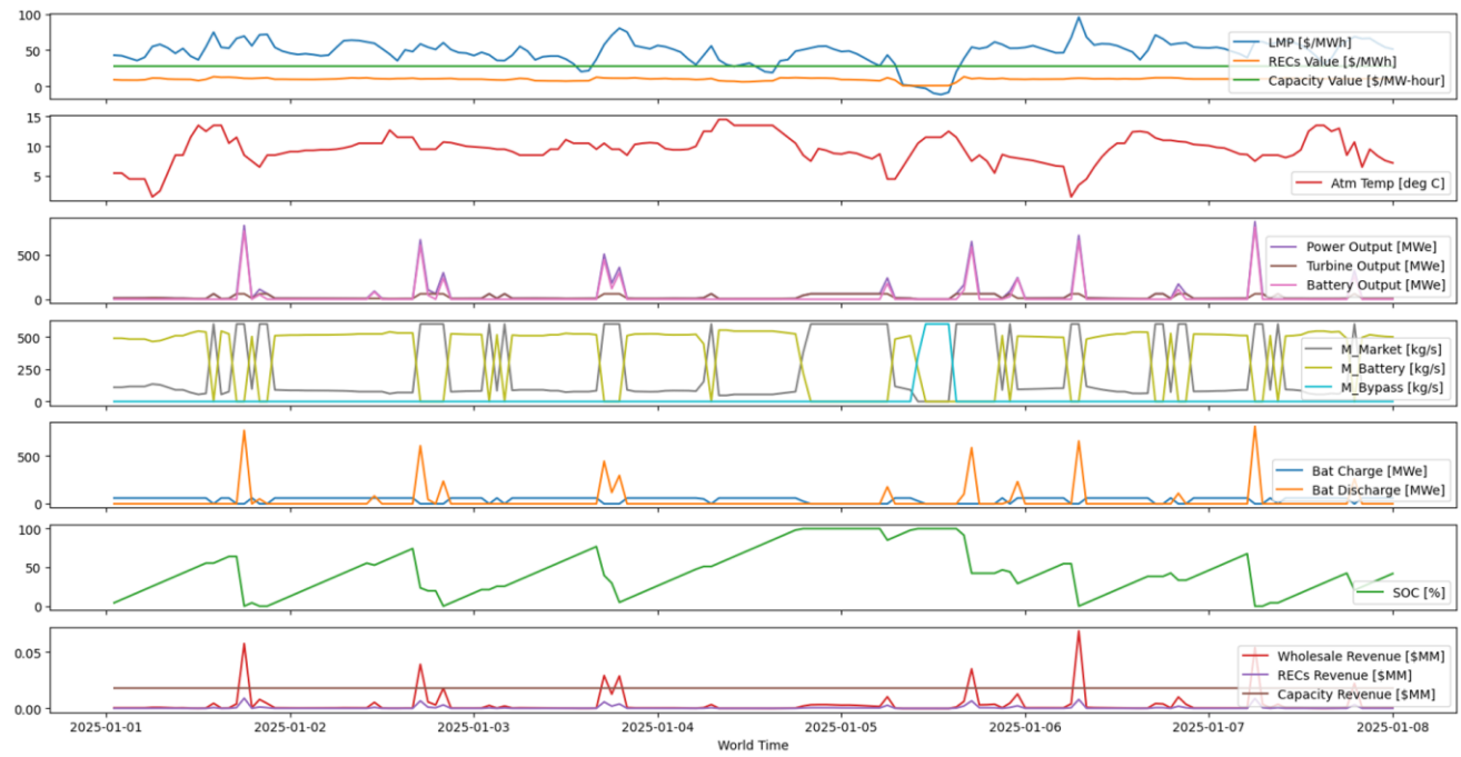
Figure 10: Hourly operational details of the bypass and battery configuration for a selected week in 2025. From top to bottom, these seven subplots show (1) market prices, (2) ambient temperature, (3) power sold to the market as generated directly from either turbine and battery, (4) geofluid mass flow rates segmentation as either used to generate power sold to the market directly (M_Market), used to generate power used to charge the battery (M_Battery), or bypassed to reinjection (M_Bypass), (5) battery charge and discharge rates, (6) battery SOC, and (7) revenue from wholesale RT, RECS, and capacity markets.
