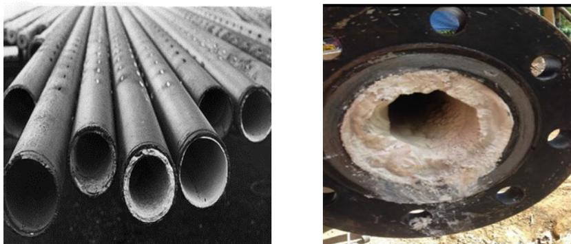
**Figure 1: Calcite scaling inside a slotted liner (left) and in a throttling valve (right) (Thorhallsson, 2019).**
