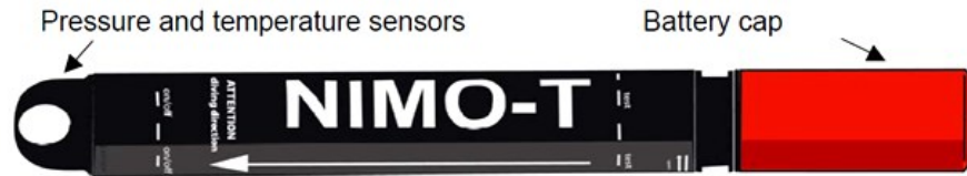
Figure 4: NIMO-T device measuring the temperature in a borehole heat exchanger (Instruction manual 2009).
