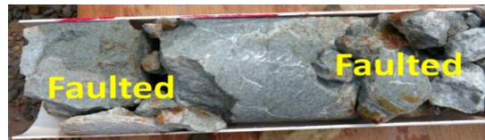
Figure 5: Core sample on faulted formation in particular depth of “DP” Well.
