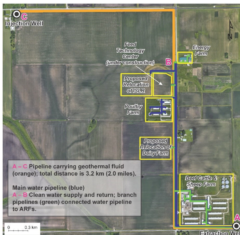
Figure 3. The piping routes for circulating geothermal fluid and clean water. The orange lines delineates the route of the main pipeline carrying the geothermal fluid between the extraction well (A) and injection well (C). The blue and green lines delineate the pipes carrying clean cold and hot water to and from the ARFs.
