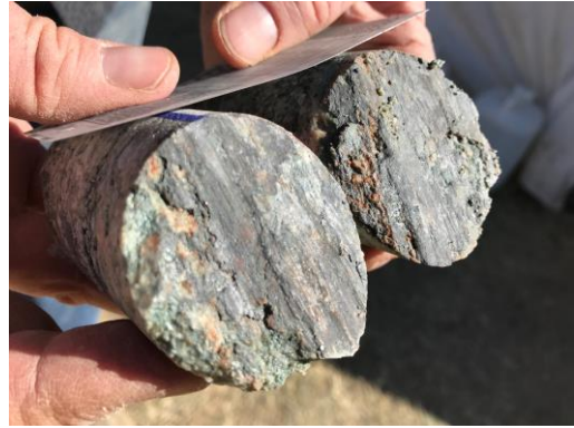
Figure 2. Slickens on fracture surface in drill core, USU Camas-1 test well.
