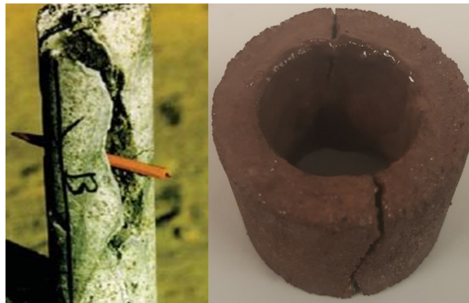
Figure 1: A typical fracture in a geothermal well (courtesy of US DOE) and a core sample after a fracture-wellbore strengthening test at the University of Oklahoma
