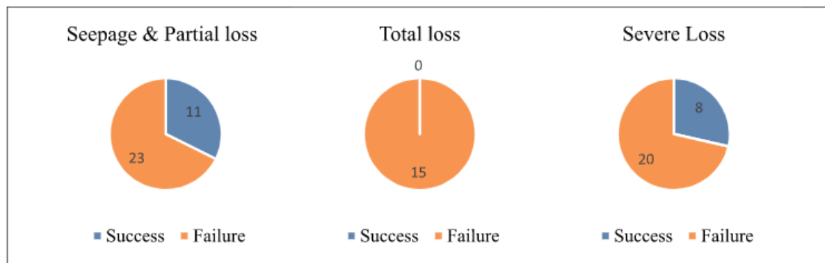
Figure 7: Using mud-mixed LCM for geothermal wells (modified after Cole et al., 2017, and Magzoub et al., 2019)
