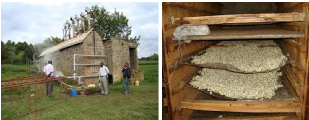
Figure 3: Geothermal energy being used by the local community at Eburru for grain and pyrethrum drying
