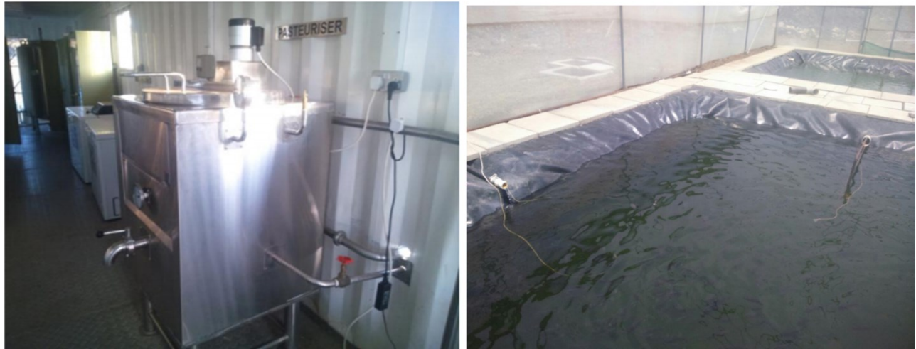
Figure 4: Geothermal Direct utilization in Menengai; Milk pasteurizer and heated fish pond (Nyambura, 2016)
