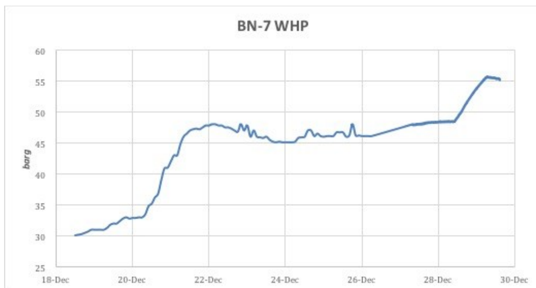
Figure 15: Well Head Pressure (WHP) of BN7 seen rising as it reacts to BN6 discharge
