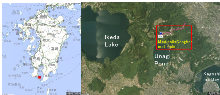
Figure 1: (Left) Kyushu island and the Medipolis geothermal field (red square). (Right) Medipolis geothermal field at the upper right. The IK-4 well is indicated by a blue dot and the ground surface geophones are indicated by red triangles. The ground surface geophone spacing is 100 m. The maps are from GSJ.
