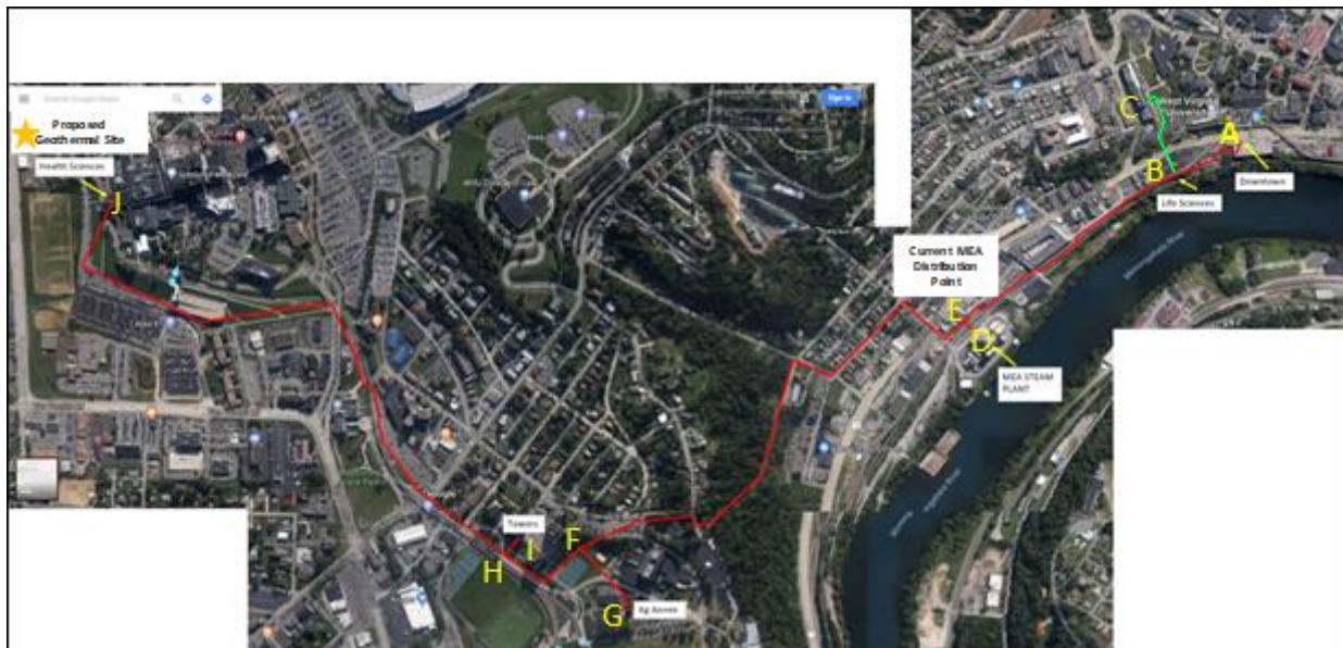
Figure 2: Google map showing the current locations of meter points and the distribution pipeline path. Pipelines in red are owned by Morgantown Energy Associates (MEA) and pipelines in green are owned by WVU. (Not to the scale).
