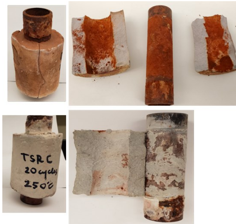
Figure 14. Appearance of OPC/SiO 2 sheath samples (top) and TSRC sheath samples (bottom) after 20 thermal cycles.
