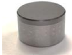
Figure 2: PDC cutter with 13.44 mm in diameter and 8 mm in thickness.
