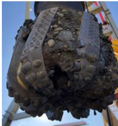
Figure 16: A photograph of Bit-C after the drilled length of 101 m where the cuttings and broken pieces of rocks stuck to most of the waterways.
