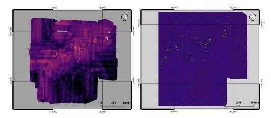
Figure 3: Unfiltered thermal map with stripes (left) being removed by FFT software (right)
