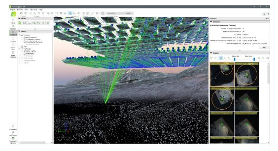
Figure 2: A 3-D perspective on how a single tie point is constructed using multiple drone images
