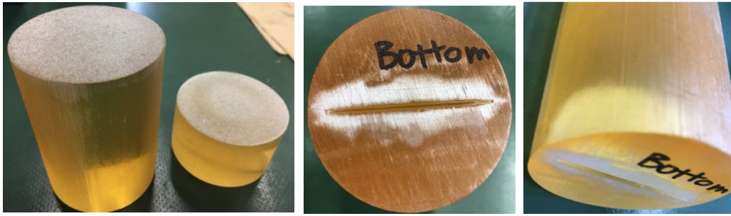
Figure 5: (Left) Ground surfaces of the cut, (Center and right) Initial crack
