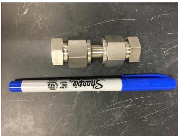
**Figure 3: Heating vessels were assembled using a 2-inch segments of stainless steel tubing with screw caps tightened on both ends to avoid solution loss caused by vaporization. 20 vessels were assembled for the 20 samples.**
