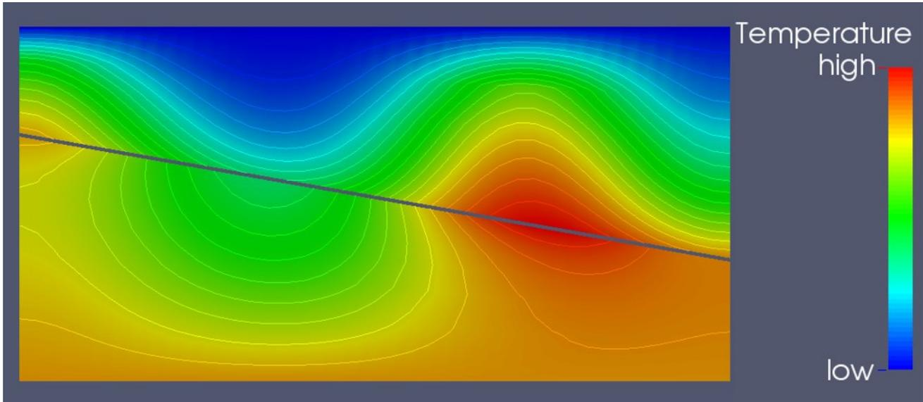
**Figure 3.2.1: The effect of shear heating on the onset of convection, observed from a transient simulation.**
