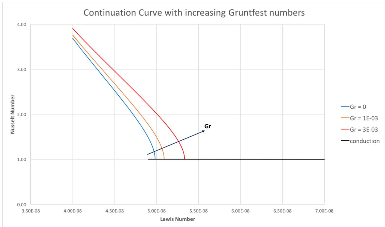
**Figure 3.3.1: Continuation curves increasing only Gruntfest numbers in identical simulations. The critical value at which convection is predicted to occur decreases as more heat (higher values for shear heating) is present in the system.**
