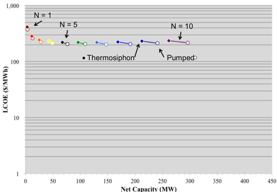
Figure 1: Levelized Cost of Electricity (LCOE) for a Carbon Dioxide Plume Geothermal System in a Reservoir with  $5 \times 10^{-14} \text{ m}^2$  permeability – Reservoir depth = 2.5 km; Geothermal gradient = 35 °C/km; Permeability =  $5 \times 10^{-14} \text{ m}^2$ .
