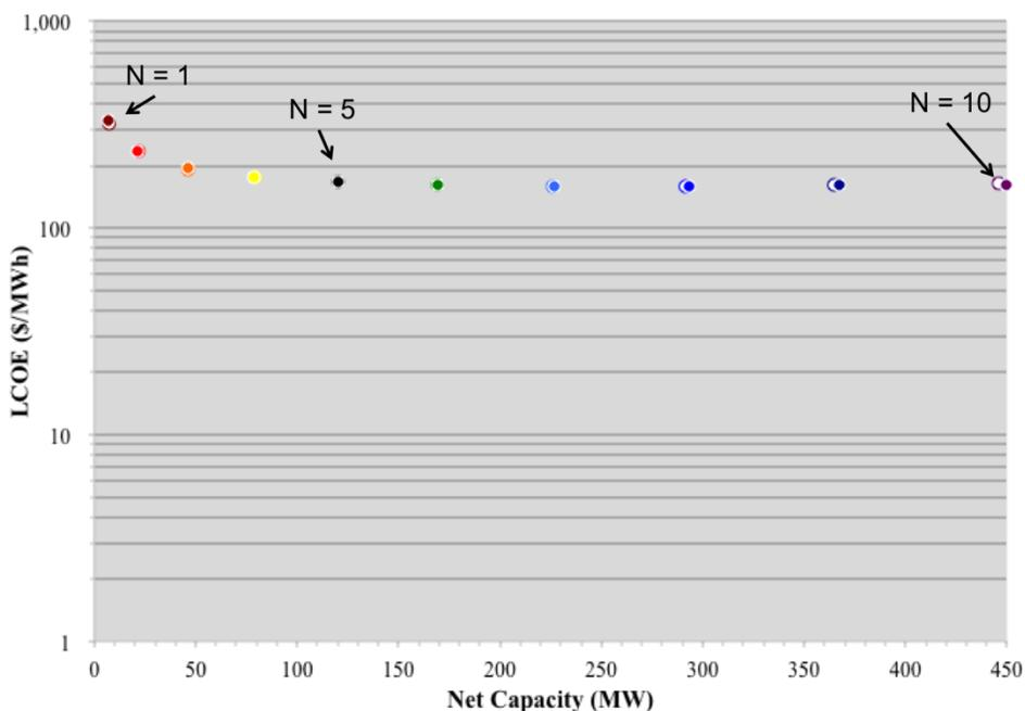
Figure 2: Levelized Cost of Electricity (LCOE) for a Carbon Dioxide Plume Geothermal System in a Reservoir with  $1 \times 10^{-12} \text{ m}^2$  Permeability – Reservoir depth = 2.5 km; Geothermal gradient = 35 °C/km
