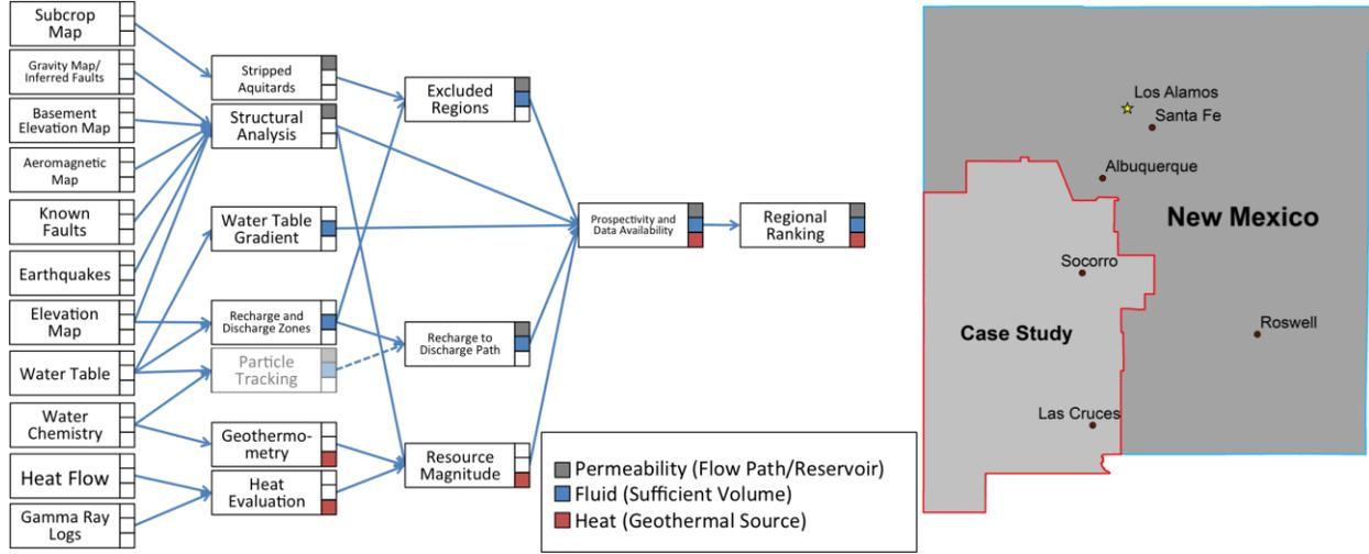
**Figure 1: The integrated framework for identifying blind geothermal prospects using the hydrogeologic windows concept. The left-most column lists the data that were used for this study. Particle tracking has been described elsewhere and is not included in the analysis here (Person et al. 2015).**
