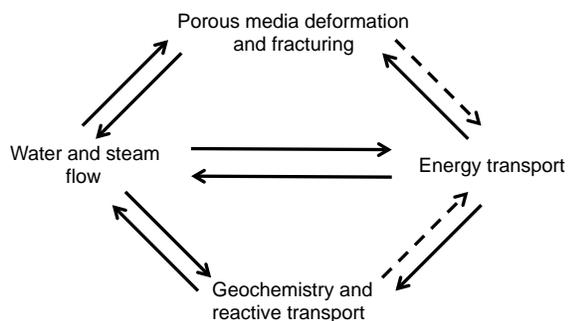
Figure 1. Strong nonlinear couplings related to geothermal systems, after Ingebritsen et al. (2008).
