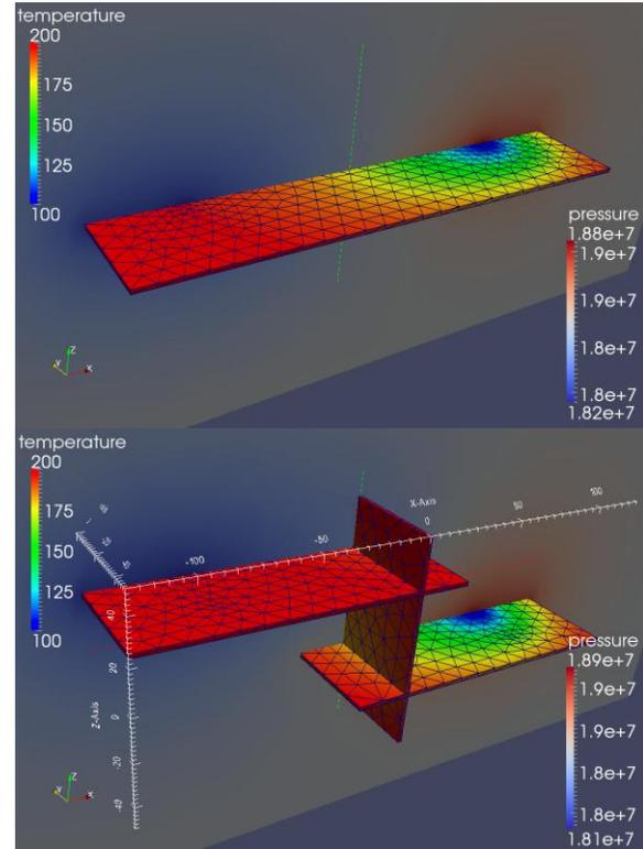
Figure 3. Temperature (in fracture domain) and pressure along the center of the reservoir matrix domain for tow simulation cases.
