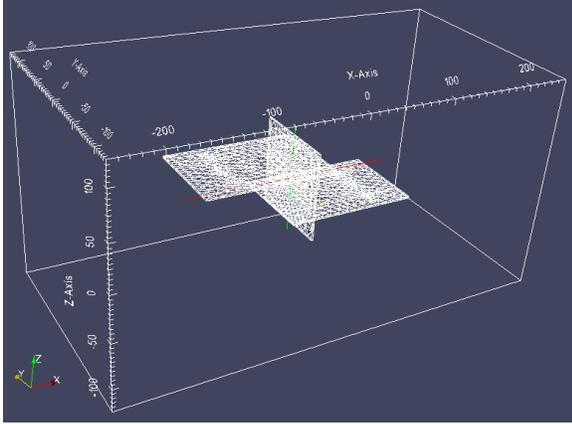
Figure 2. Three-dimensional mesh for the simplest fracture flow problems under consideration.
