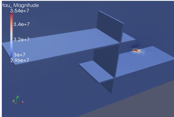
Figure 4. Early-time stress magnitude change in the vicinity of the injection horizon within the simulation domain.
