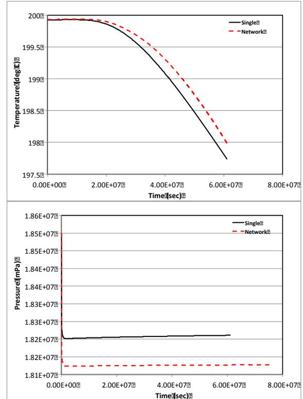
Figure 5. Comparison of produced fluid temperature and pressure for the simulation cases shown on Figure 3.
