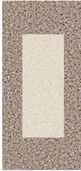
Figure 3-8. 3D diffusion model. The sample surface of the model is fully open thus diffusion can be in any direction into the sample.
