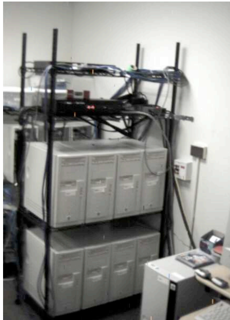
Figure 4.1: A 16-node Beowulf PC cluster built in the Geophysics Department at Stanford University.
