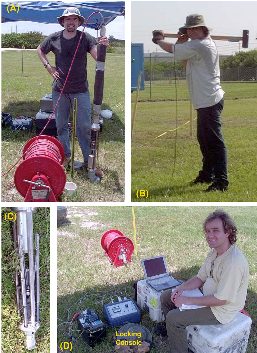
Figure 3.15: VSP Seismic System : single level locking 3-component downhole receiver (A), sledgehammer source (B), lever locking mechanism on the 3-component tool (C), (D) VSP surface control setup
