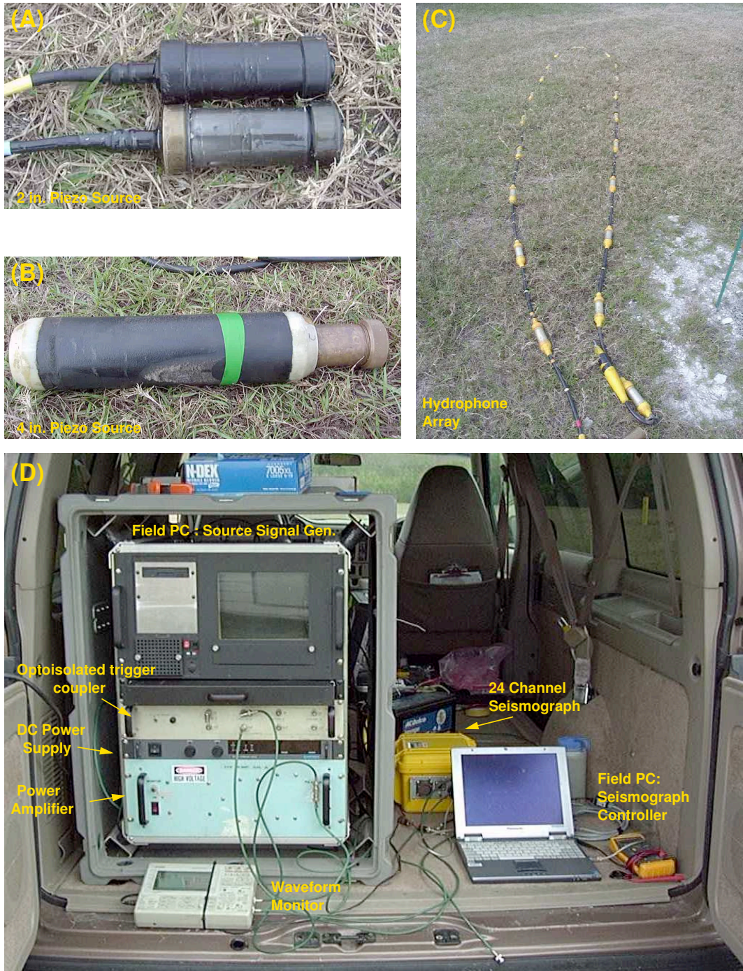
Figure 3.9: LBNL Crosswell Seismic System : (A) 2 in.piezoelectric sources, (B) 3.5 in. piezoelectric source, (C) 24 channel hydrophone array, (D) Source electronics rack and recording system.
