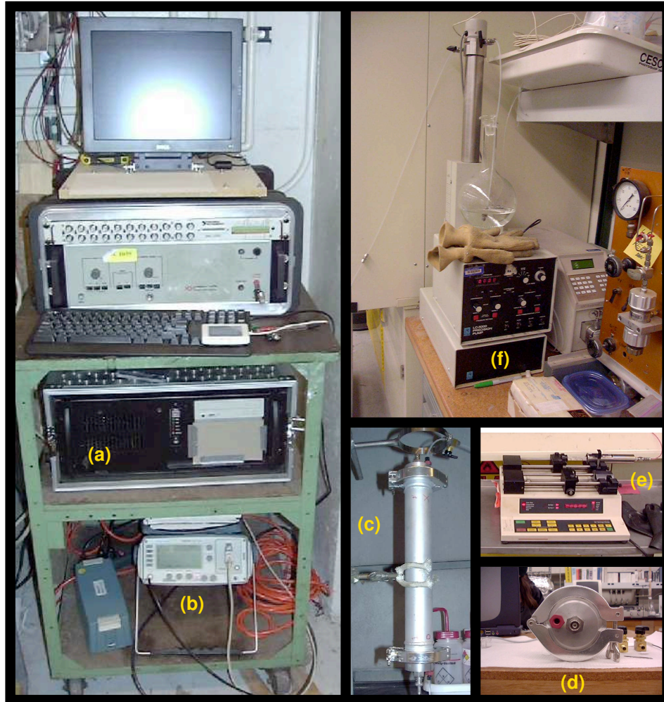
Figure 5.3: Primary Components of the TDR System : (a) Lab computer used for data acquisition, (b) Tektronix 1502B TDR, (c) Coaxial sample holder used for dielectric measurements, (d) Close up of coaxial end-cap showing BNC connector and PEEK flow port, (e) Harvard precision syringe pump used for TCE injection, (f) ISCO precision pump used for water saturation process
