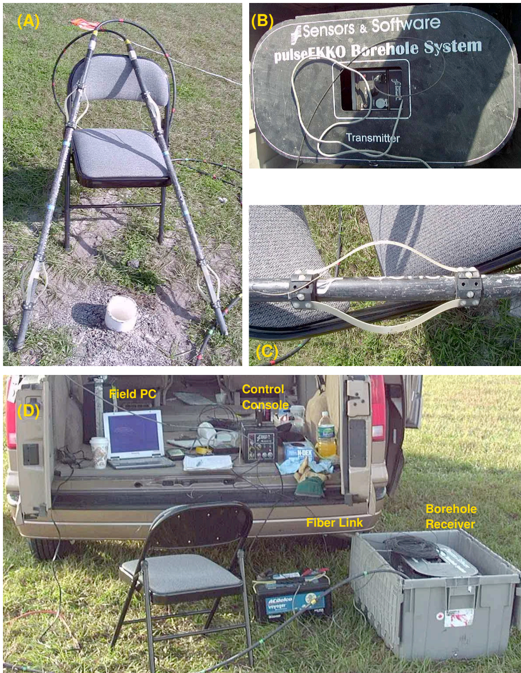
Figure 3.12: Crosswell Radar System : The Pulse-Ekko 100 borehole GPR system, (A) 200 MHz antennas with borehole centralizers, (B) transmitter unit with Farraday cage, (C) close-up of borehole centralizer, (D) control equipment
