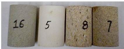
Figure 6: Four rock samples (1 Boise sandstone, 1 chalk, and 2 Berea sandstones) used in this DARS experiment.
