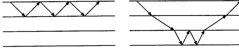
Figure 1.1: When perturbation parameters is not small, the recursive relation is not valid because of unobservable reflections.
