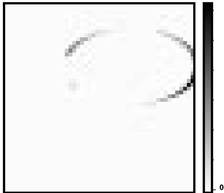
Figure 4.45: Gradient of permeability field with respect to the ellipse semimajor axis: multiple objects.
