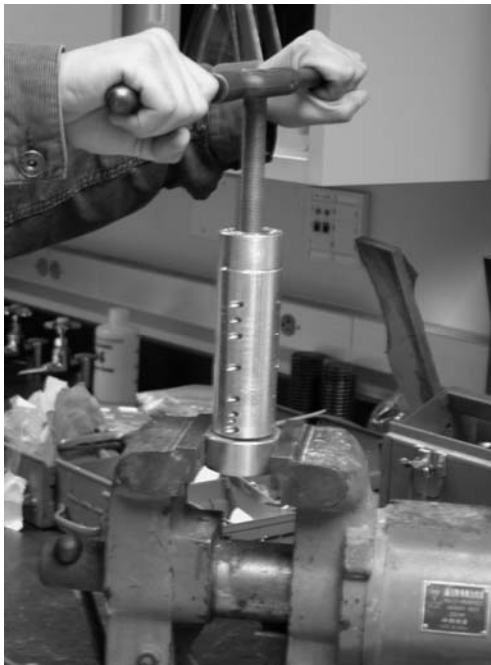
Figure 3-5: Preparation of the core using the coal press.
