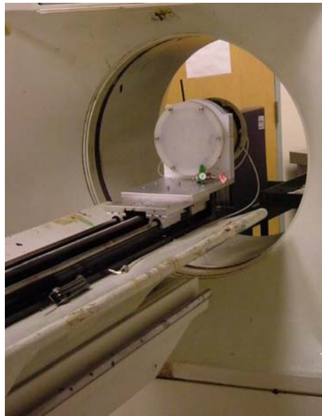
Figure 3-11: Imbibition cell on the positioning system.
