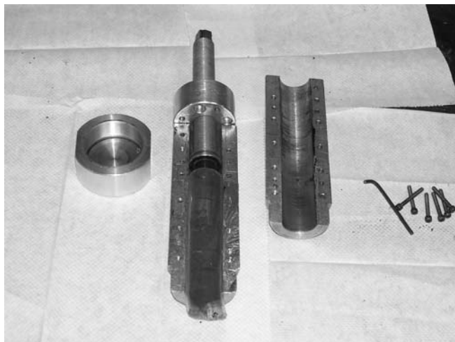
Figure 3-4: The various parts of the coal press.
