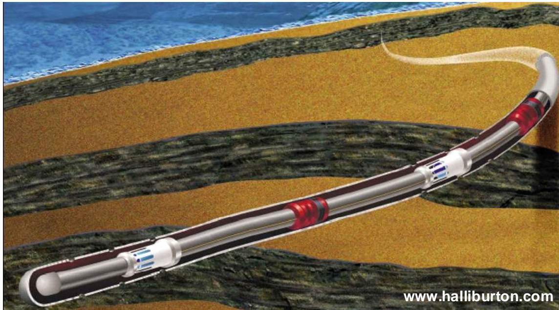
Figure 1.1: Typical smart well penetrating multiple productive zones.
