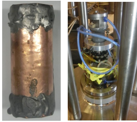
Figure 2: Sample in copper jacket (left) and in the cell (right).
