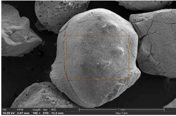
Figure-2: SEM image of 10/35 petroleum coke proppant with EDX analysis showing elemental composition.
