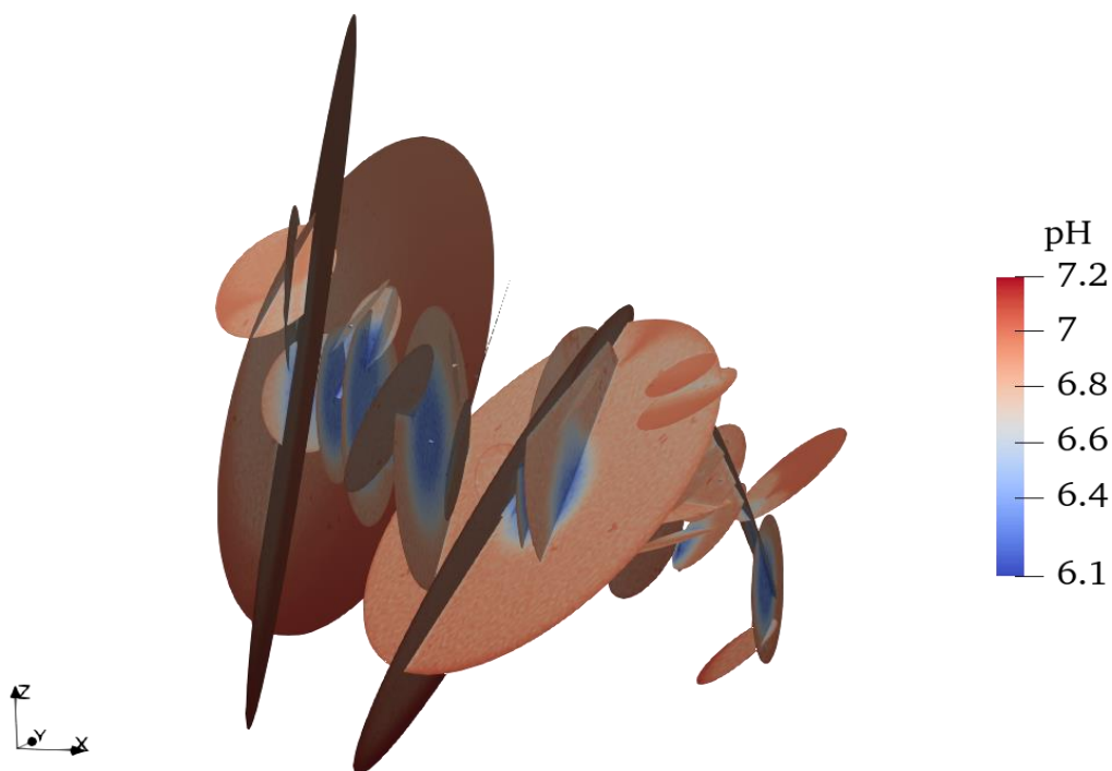
Figure 4: pH profile in DFN after 1 year of circulation test. The increased acidity shown in blue around the injection wells can be attributed to temperature-dependent changes in the activity of H^+ ions.
